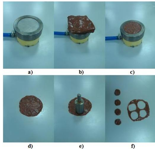
Figure 2: The steps of the sample preparation.
